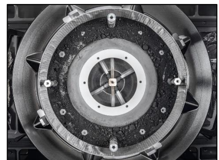
A top-down view of the TAGSAM from OSIRIS-REx, with the lid removed to reveal the remainder of the asteroid sample inside.
